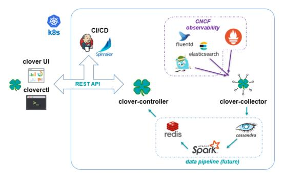
The diagram above shows the flow of data through the visibility services where all blue arrows denote the path of data ingestion originating from the observability tools. The **clover-collector** reads data from these underlying tools using their REST query interfaces and inserts into schemas within the **cassandra** data store.
